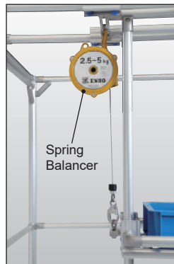
2 Using the Spring Balancer to hold the Z-axis direction at any height.
