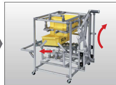
3 When return the handle, the lowest container will be discharged from the table, and the bracket stays in the position of holding the next container.
