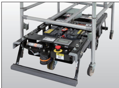
1 The AGV sneaks under the trolley.
