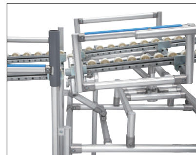
3 Stopper module (rotation) will completely unlock after table finished rotating and the container will be discharged.
