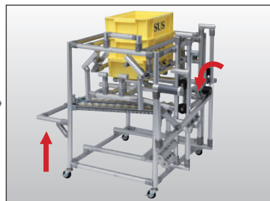
2 Push the handle down forward and table will go up to lift the container in the lower level. At the same time, the bracket that hold the container will spring up.
