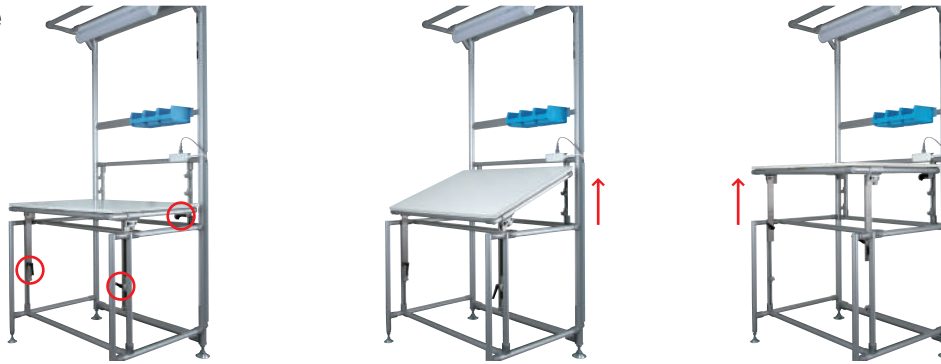
Unlock the handle (3 places) under the table to adjust the height of the table. (Height adjustment 200 mm)
