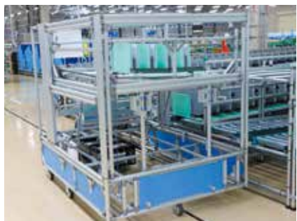
Shown here with table raised, the AGC battery provides power for motorized up-down movement.
