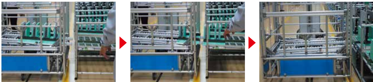
The AGC complying with its program conveys the full tray loaded from the chuter in the floor to the assembly process and ejects the recovered tray. When the cart is empty, the table tilt changes.
