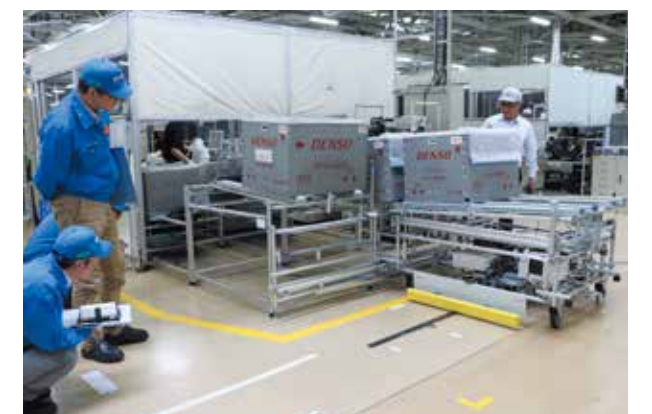
Excerpt from AGC (Automatic Guided Cart) interviewed in the Sing 33 issue (Japanese version only). A mechanism to automatically handover the workpiece by way of a Karakuri mechanism was introduced.
