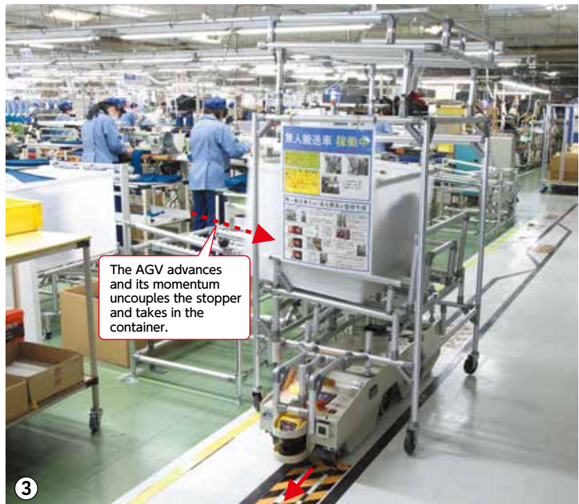
Once the sewing process is ready, turning on a switch runs the AGV cart. A mechanism links the cart and chuter together to automatically deliver containers. The cart goes back and forth between the sewing process and the assembly process up to four times per hour.
