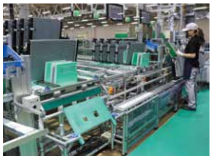
View of the assembly process. Worker starts assembly using the workpiece supplied from the upper rack and ejects the now empty tray to the lower rack.
