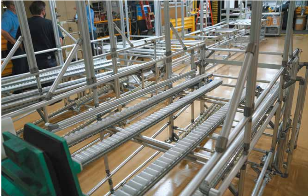
The shooters are for a line that assembles radiators and fan shrouds.
