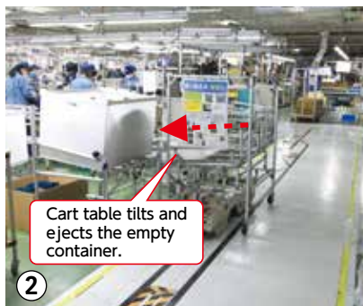
Once the sewing process is ready, turning on a switch runs the AGV cart. A mechanism links the cart and chuter together to automatically deliver containers. The cart goes back and forth between the sewing process and the assembly process up to four times per hour.
