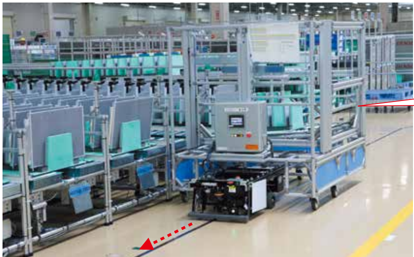
Shown here with table raised, the AGC battery provides power for motorized up-down movement.
