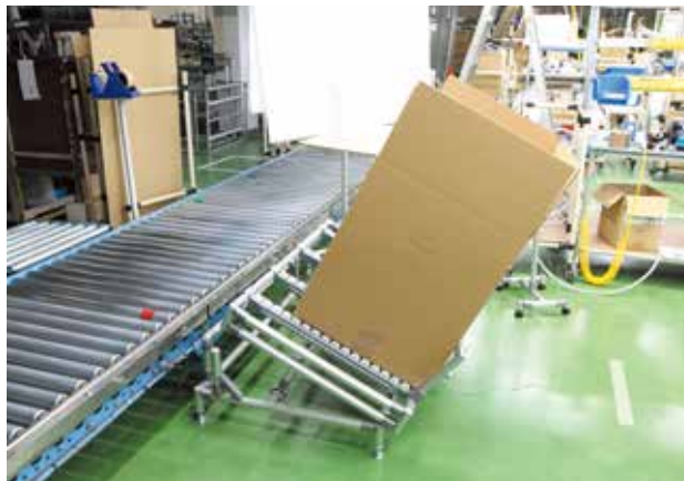
A see-saw type table capable of easily inserting the finished chair by tilting toward the worker side and returning it to the conveyor by lifting up from the front when packing is finished.
