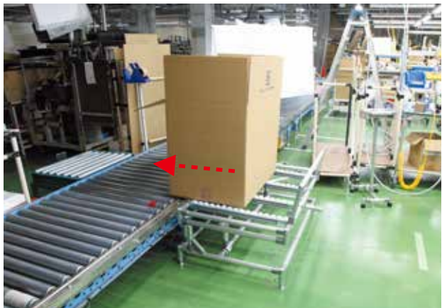
A see-saw type table capable of easily inserting the finished chair by tilting toward the worker side and returning it to the conveyor by lifting up from the front when packing is finished.
