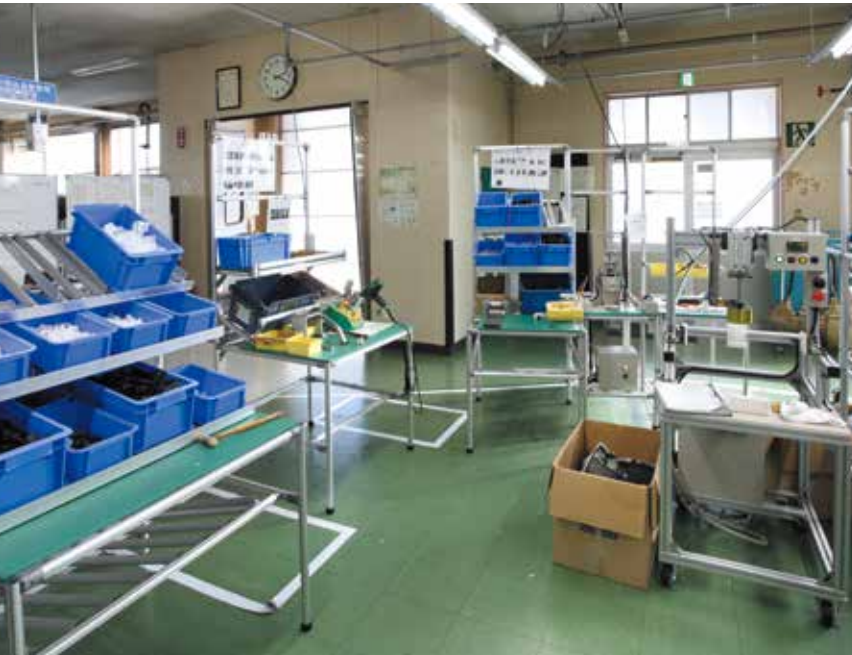
A parts shelf of a work table installed to tilt so the operator can easily take it out. Parts are supplied from outside to the line, and then the emptied containers are ejected from the feet.
