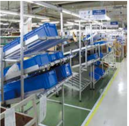
A parts shelf of a work table installed to tilt so the operator can easily take it out. Parts are supplied from outside to the line, and then the emptied containers are ejected from the feet.
