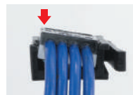
Bad example(1) Insufficient cover push in.
