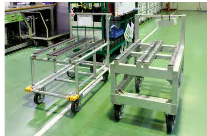
GF cart (left) and SF cart (right) actually used in the process. The GF cart in the photo is a partially modified version of the equipment which was requested to SUS to assembly for the first time, with a load capacity of 320kg.
