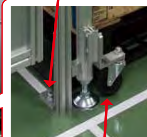
In order to carry in and out material from the back shutter, casters were attached to all the foot suspensions, making it movable.
