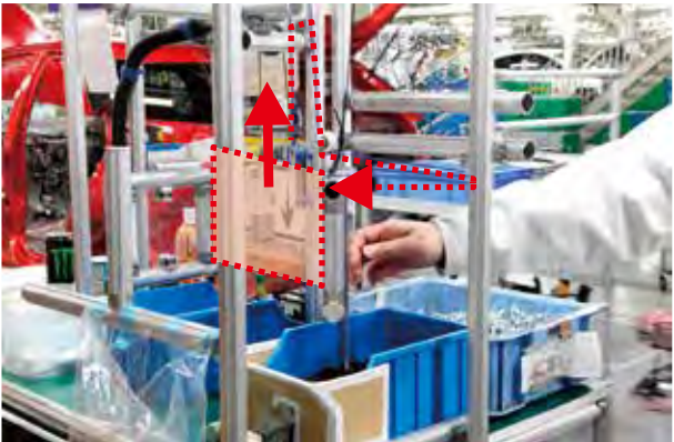
This is a new karakuri made after the exhibition. Two doors are installed in front of the two types of parts placed on the workbench. The door on the back will not open, unless the door in the front is pressed, preventing unattached parts from being left unattached.
