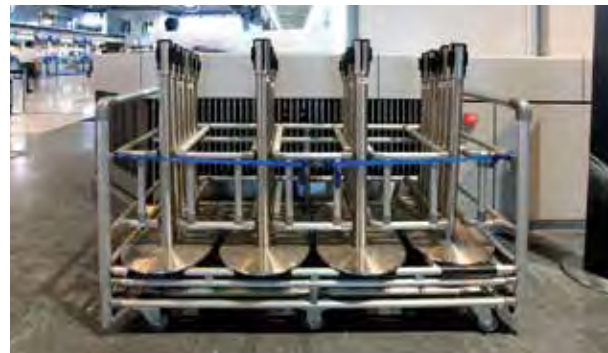
Since the stacking style tape stanchions are slightly inclined by stacking them, a frame for supporting the column is attached, so that it does not collapse even if it shakes.
