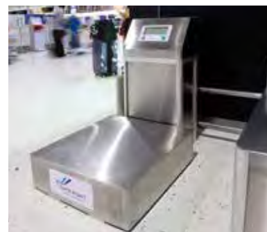
A prototype of the weighing scale delivered just before the interview. It is based on a ready-made scale that was originally in use.
