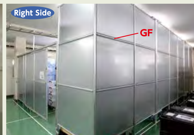
In order to secure a passage for visitors, we produced the partition, which was previously made from plastic corrugated cardboard, with GF and AZ using aluminum composite board. Because it is lightweight, looks good, and has a sense of unity, it is highly appreciated by other departments and people in other processes.
